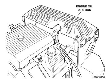
Figure 7-4. Engine Dipstick Location
